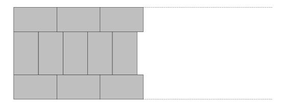
I lay the slabs lengthwise along the edges of the path and crosswise in the centre of the path, as shown in the diagram. When I have placed the final slabs in the pattern, I can, if necessary, make a single straight cut across the end of the path with my chainsaw, in order to leave an exactly rectangular paved area.
