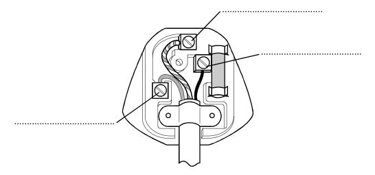
(b) (i) Explain how the earth wire and the fuse protect a person from an electric shock when there is a short circuit to the metal case of an appliance.
